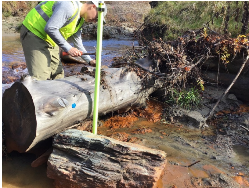
Figure 3. Stone staff tagging and collecting GPS locations of wood at monitoring station WR3.
