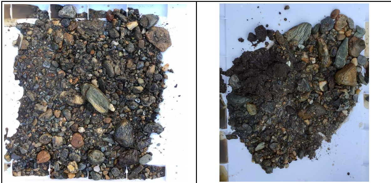
Figure 6. Photographs of the sediment below the surficial armor layer at Site 101 (left photo) and Site 102 (right photo).
